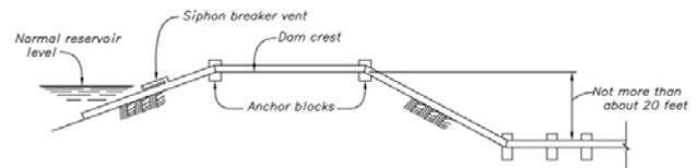
**Figure 4. A simple siphon constructed over the crest of an embankment dam. [1]**
