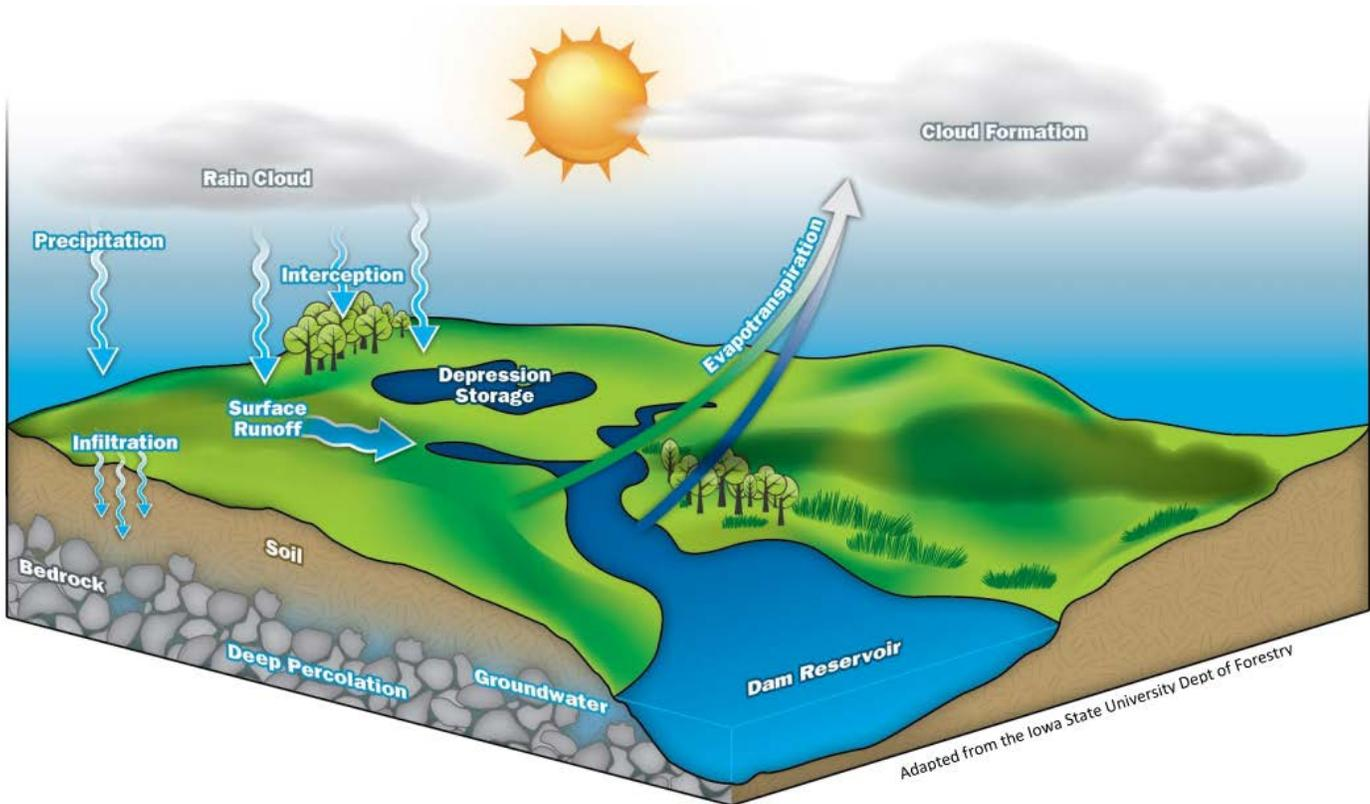
Figure 1. Total rainfall-runoff process with losses
