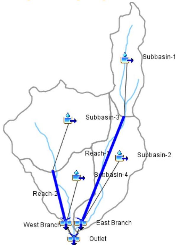
**Figure 2. Schematic of typical HEC-HMS watershed model[5]**
