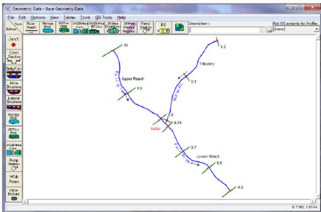
Figure 3. Example of 1D HEC-RAS model geometry [4]
