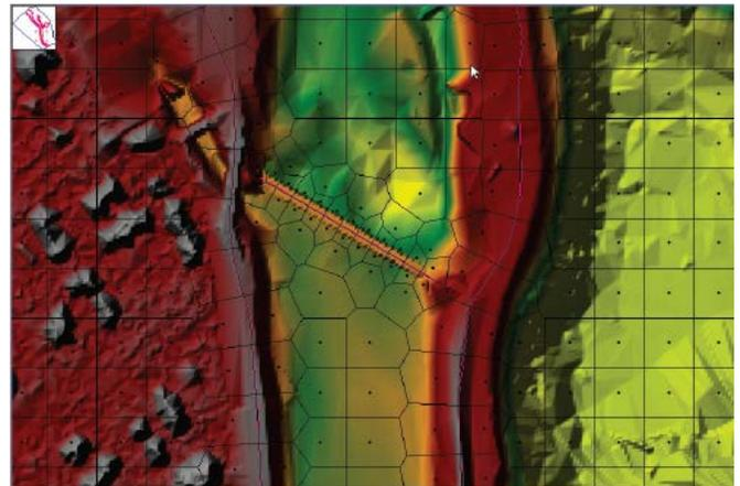
Figure 4. Schematic of typical 2D HEC-RAS computational mesh. [4]
