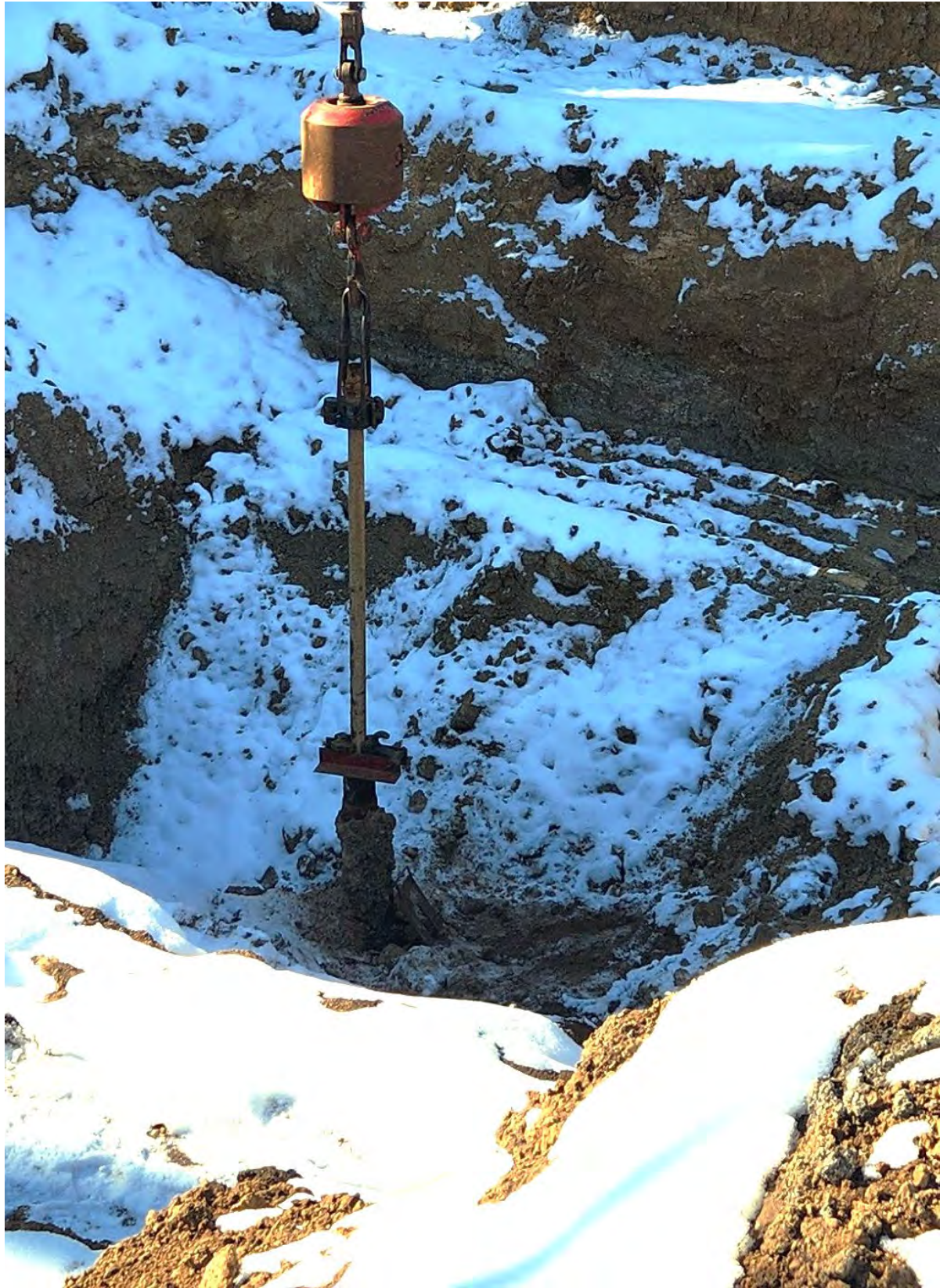
String pull - 15,000 pounds – no more upward movement – no downward movement
