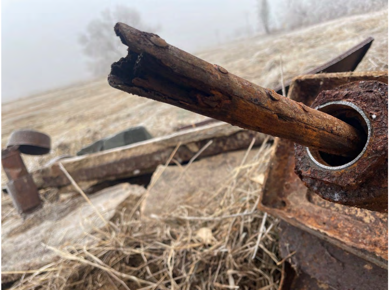
Photo 4 – Column Pipe and Windmill shaft broken below head – see clean steel break
