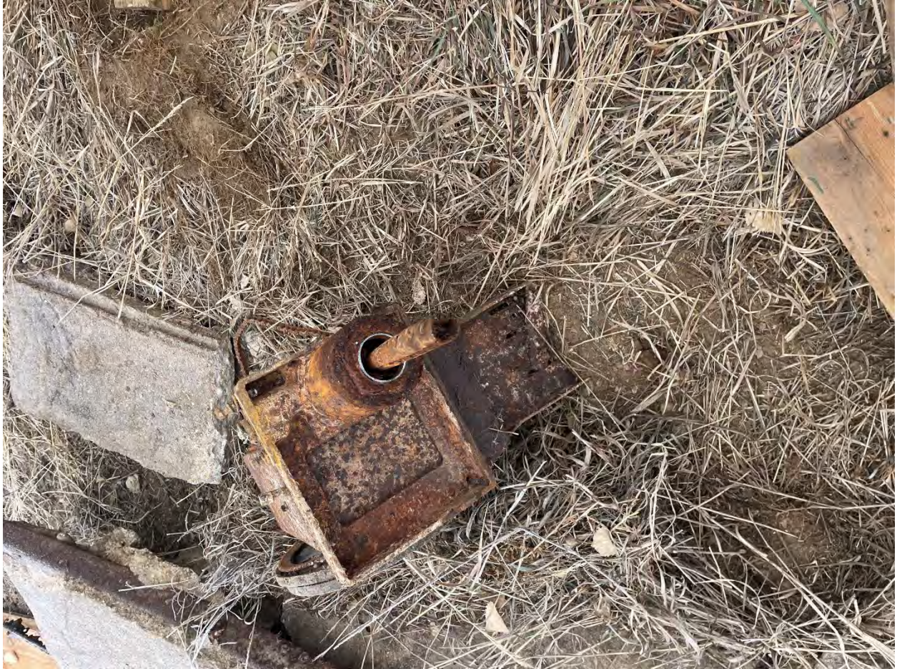
Photo 3 – Column Pipe and Windmill Shaft – Both Broken
