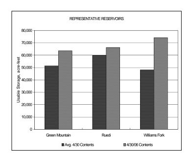
The SWSI value of +0.7 indicates that for April the basin water supplies were slightly above normal. Flow at the gaging station Yampa River at Steamboat was 1025 cfs, as compared to the long-term average of 586 cfs. The overall snowpack for the Division was 84% of average.
