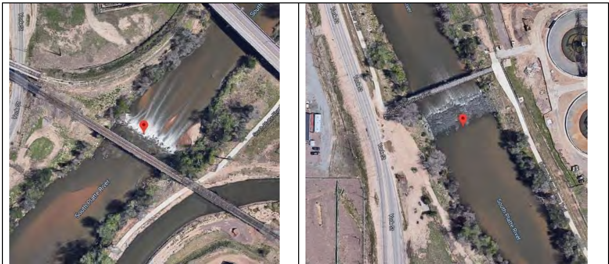
Figure 3: Examples of Grade Control Structures. Photo Credit Google Maps
