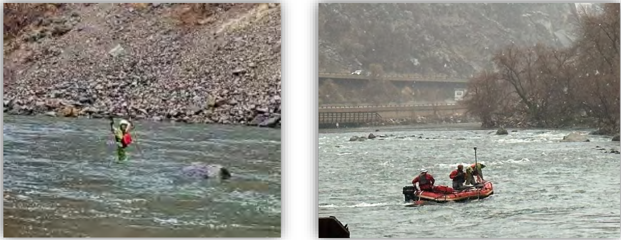
Figure 2. Survey Methods. GNSS rover (left) and boat mounted GNSS integrated SBES (right)
