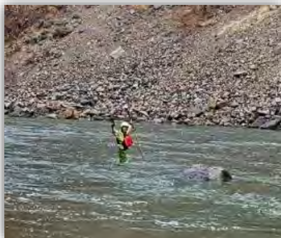
Figure 2. Survey Methods. GNSS rover (left) and boat mounted GNSS integrated SBES (right)
