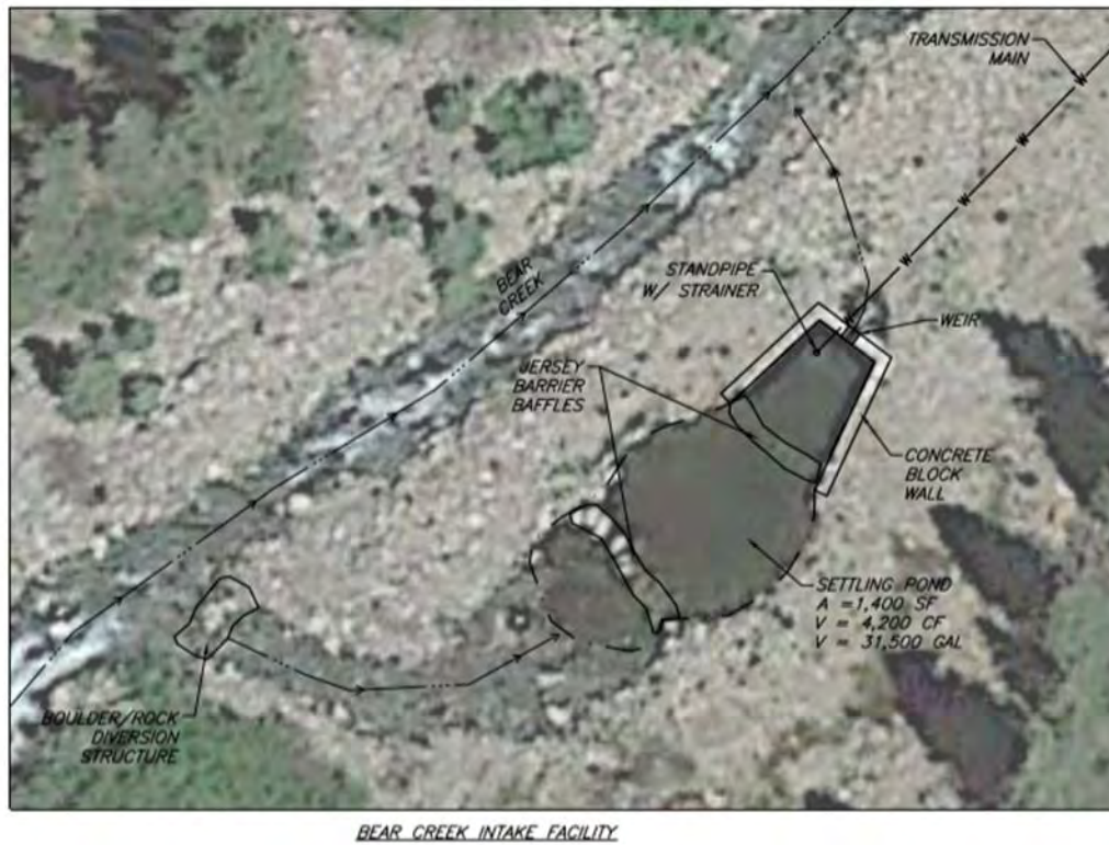
Figure 3-13 Schematic of Bear Creek Intake
