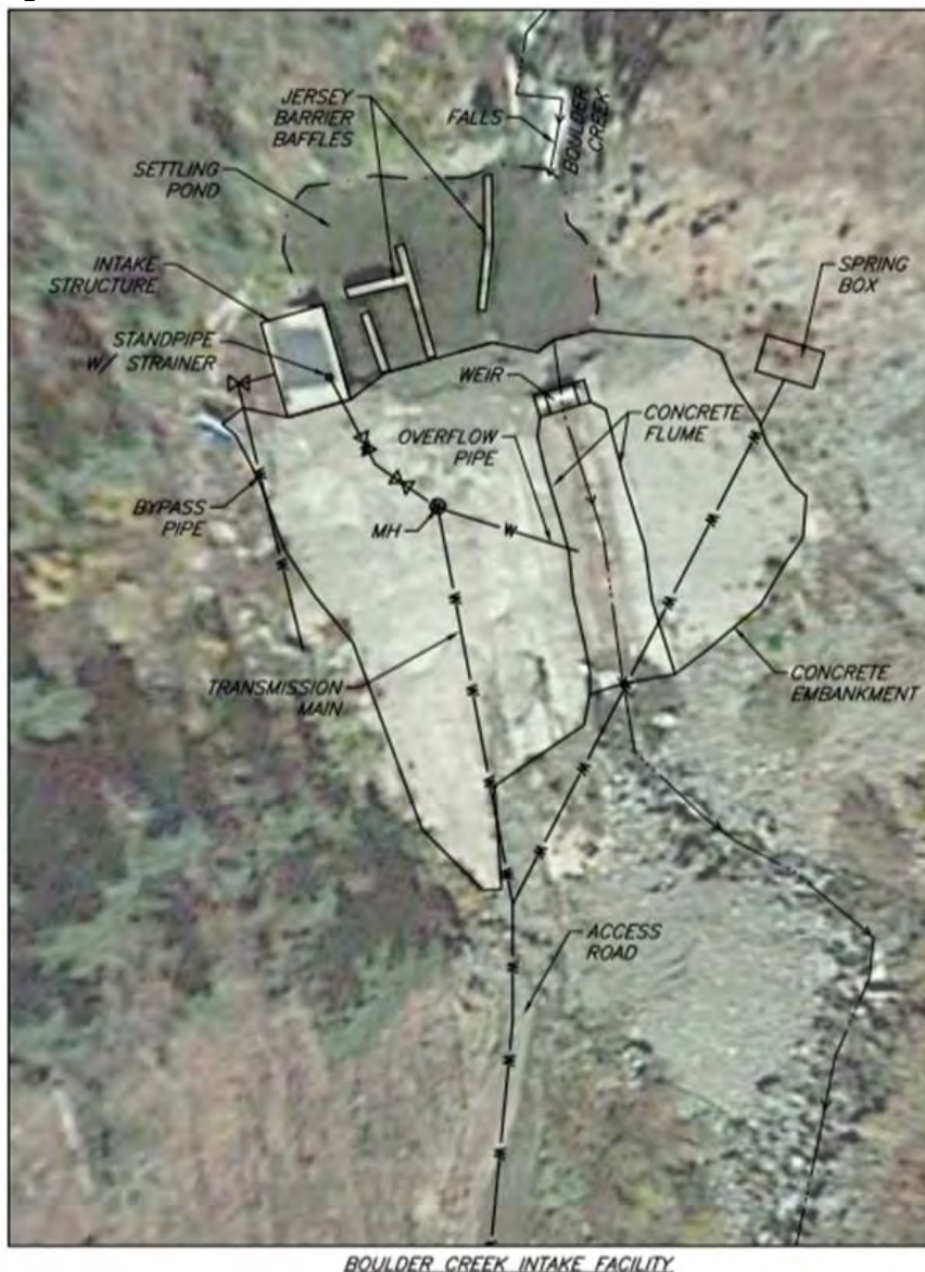
Figure 3-12 Schematic DWG of Boulder Diversion and Intake
