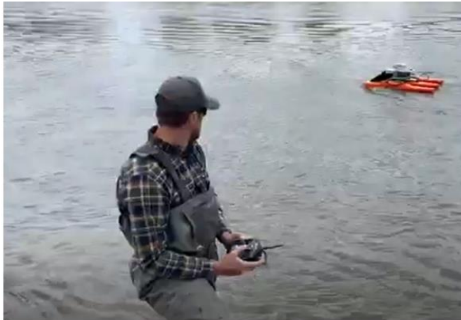
Remote-controlled Automatic Data Collection Platform (ADCP) system developed by DWR to expand use and improve safety of ADCP's
