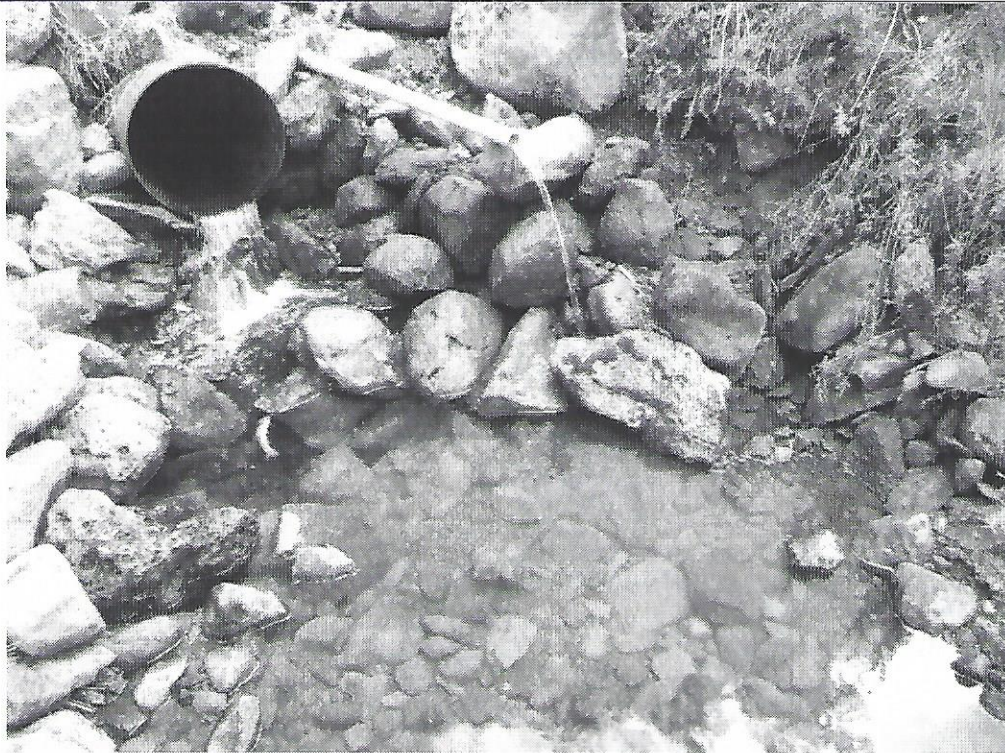
Photos 8 & 9 View looking upstream and across at outlet pipe and seepage collection pipe with visibly dye; Time approx. 20 minutes
