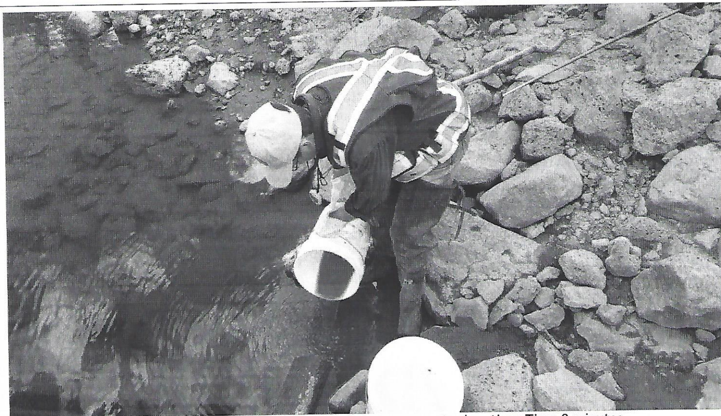
Photo 4: Introducing dye into suspected seepage entry location; Time 0 minutes.
