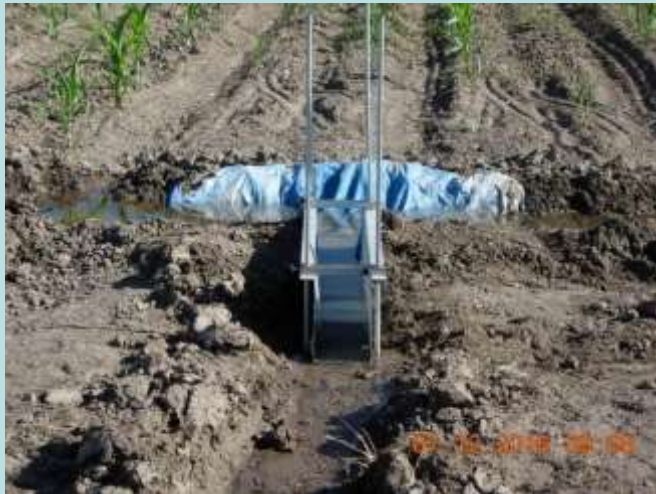
Field inflow meter and RO ramp flume
