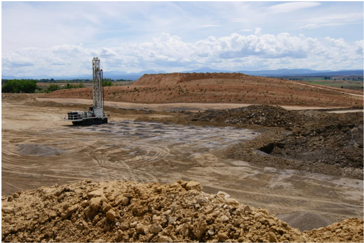
Photo 3 – Drill rig and pattern of holes
