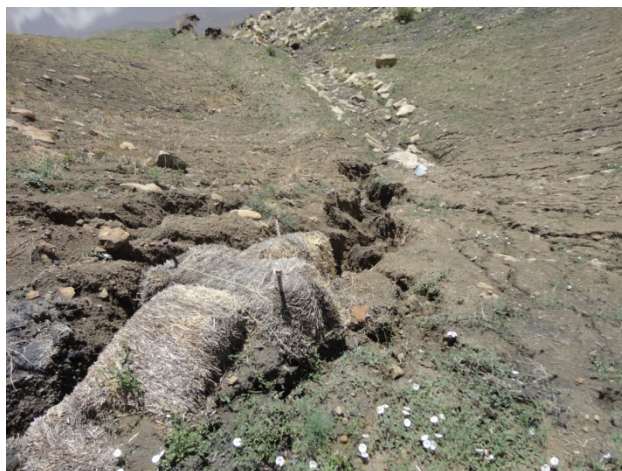
Photo 40: Large gully below conveyor, above pond 8
