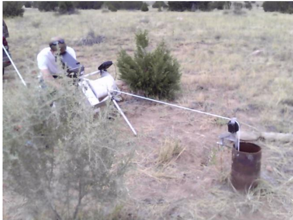
Photo 1: investigation of MW-NW with bore hole camera.
