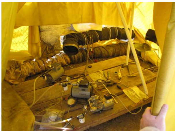
Photo 5 – Heated Tent with Air Pumps
