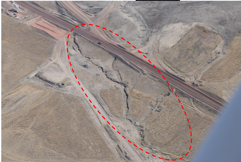
East Pyeatt re-established drainage north of life of mine road near Parcels A-B-98 and A-B-96. Channel appears incised.
