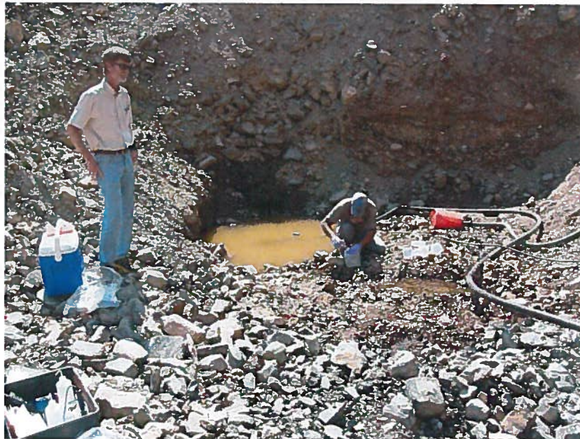
Photo 7 – Operator's representative (center of photo) collecting sample where water flows to low area in grout curtain area. Black pipe on right side of photo carries water from pump in pool to water treatment plant approximately 400 feet away.
