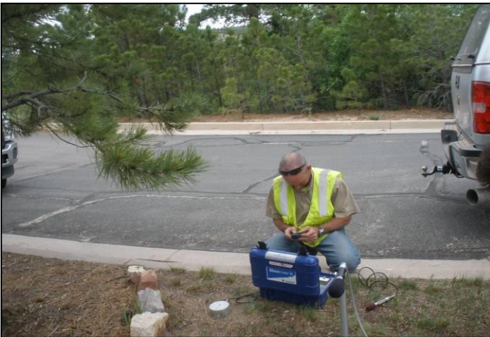
Figure 3 Randy Morris of Buckley explosives (operator's consultant) setting up the blast monitor prior to blast.
