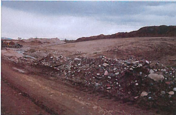
View, facing east, toward the active mining face in Mine Cell B. The mined slope on the right side of the photo has been graded to 3H:1V or less. A topsoil stockpile is located at the rim of the graded slope.
