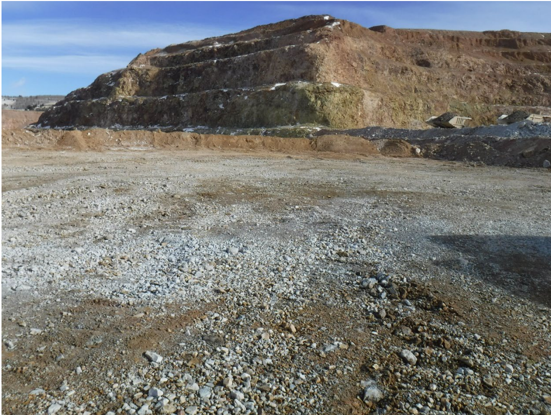
Photo 19: Schist Island backfill, high compaction "rind" foreground and low compaction material near haul trucks
