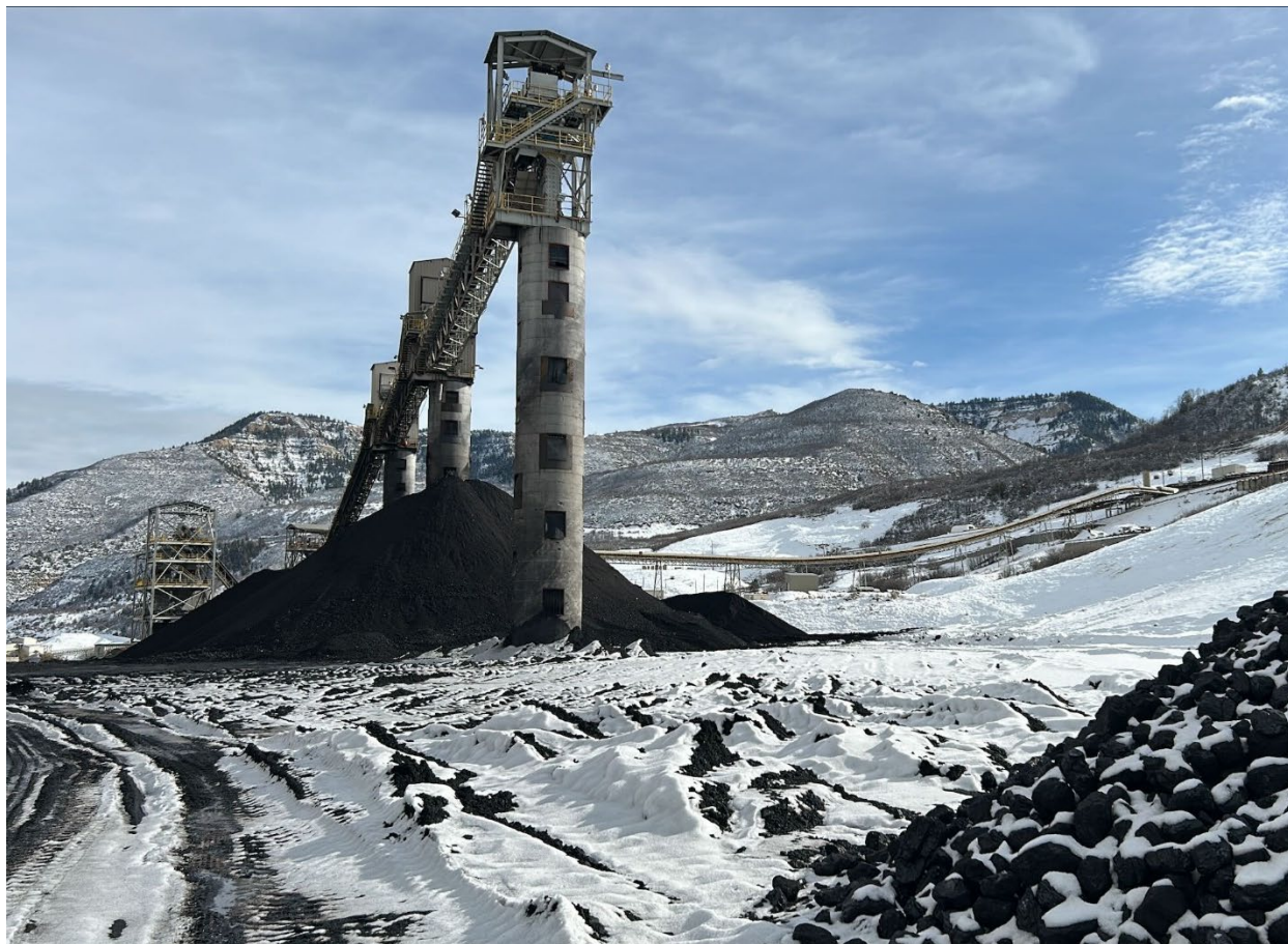
Figure 9: Run-of-Mine coal stockpile pad from west, showing fines completely removed
