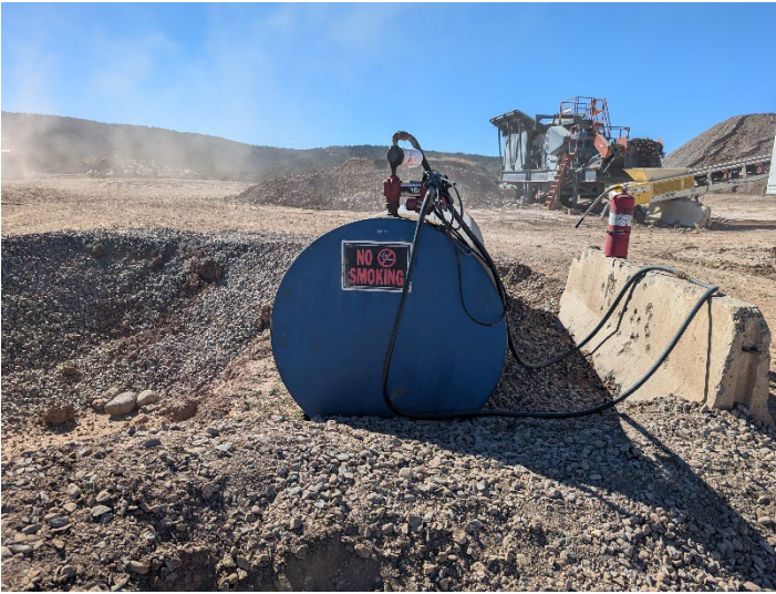
Fuel tank lacking secondary containment
