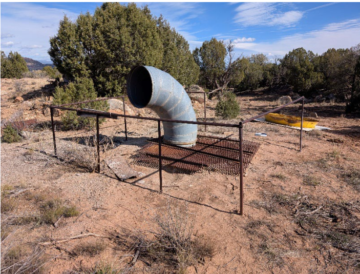
Ventilation fan shaft – fan removed, shaft not yet secured
