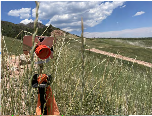
4. GRASSES ESTABLISHED ON SLOPES. OCCASIONALLY BLOCKS PRISM DURING READINGS.
