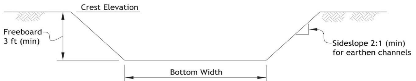
Spillway Section
