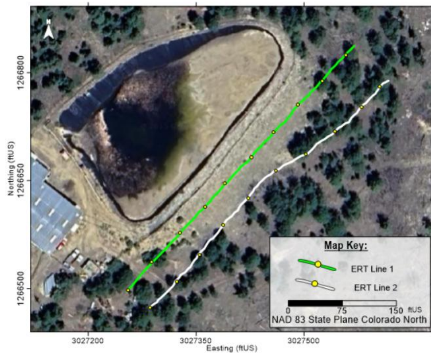
Figure 2. Shows the Tailings Pond at the Gold Hill Mill site with the locations of the two electrical resistivity lines collected on July 8 th , 2025.
