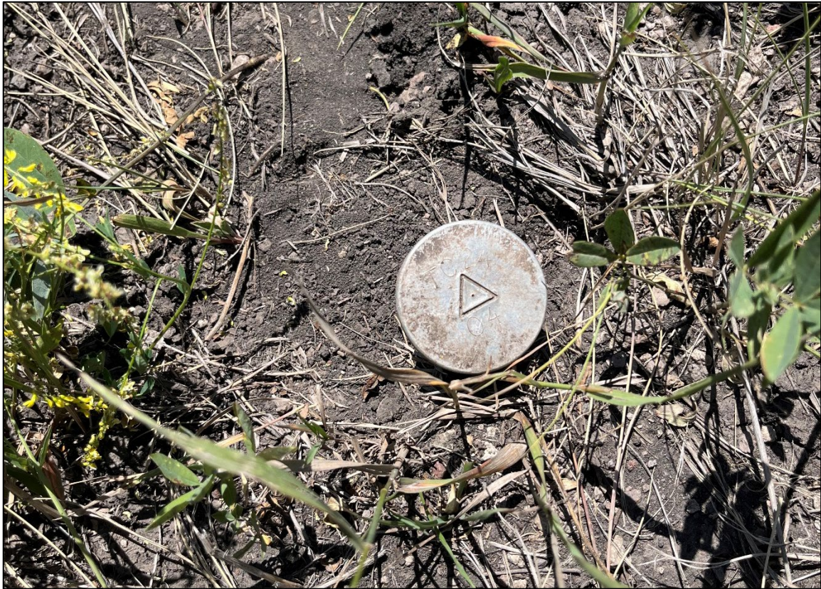
Photo 4: Abandonment marker for drillhole TC24-04.
