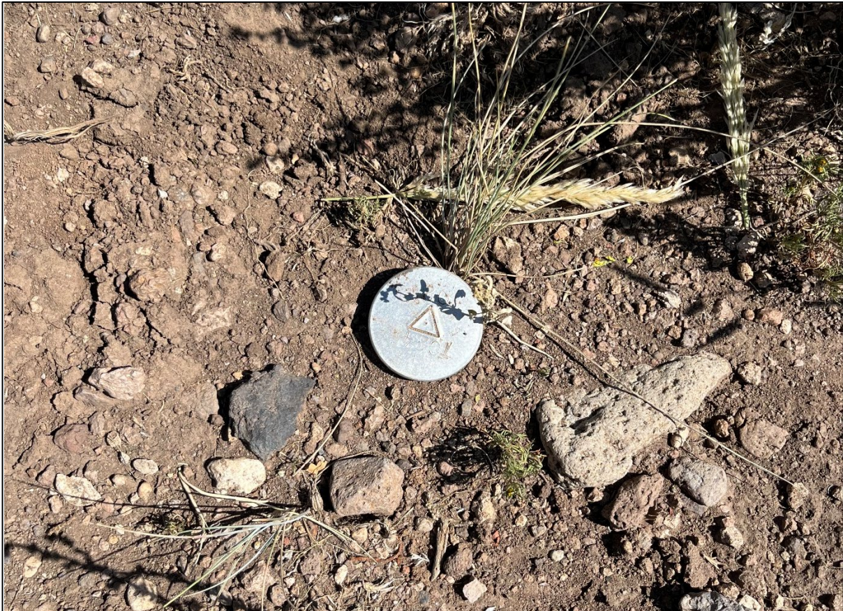
Photo 3: Abandonment marker for drill hole TC24-02.
