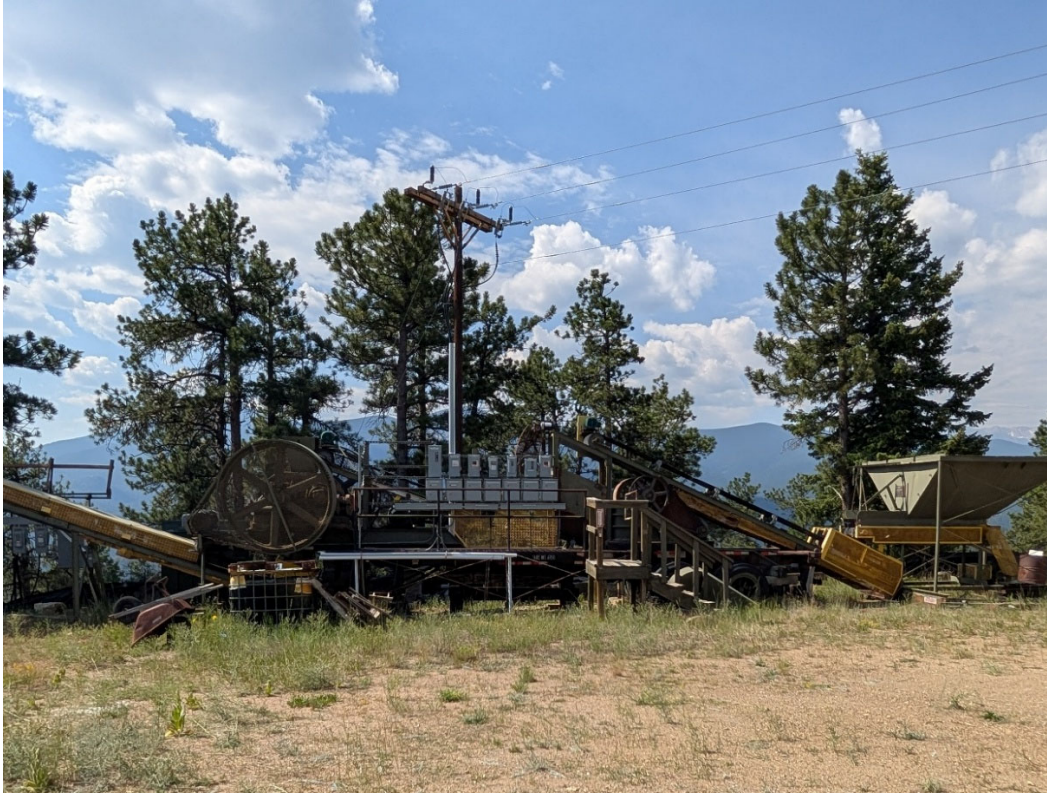
Photo 3: Looking south at the crusher feed bin, crushing plant, and conveyor.
