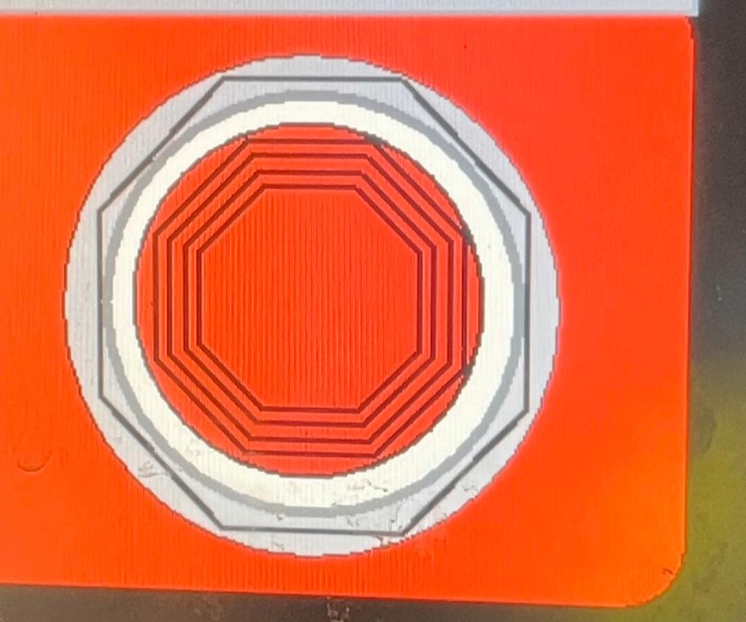
THE E-STOP BUTTON HAS BEEN PRESSED. POWER IS NOT FLOWING TO THE INPUT/OUTPUT CARDS. PULLING OUT THE E-STOP AND PRESSING THE SYSTEM RESET BUTTON WILL RETURN THE SYSTEM TO NORMAL.
