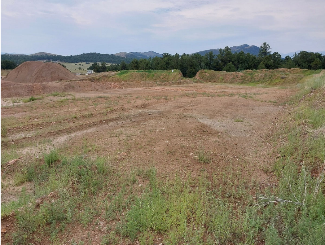
Photo #7: View of the current mining area with the topsoil stockpile along the back with the stormwater break in the berm and the topsoil sign visible. The stockpile of product material can be seen in the background on the left side of the picture.
