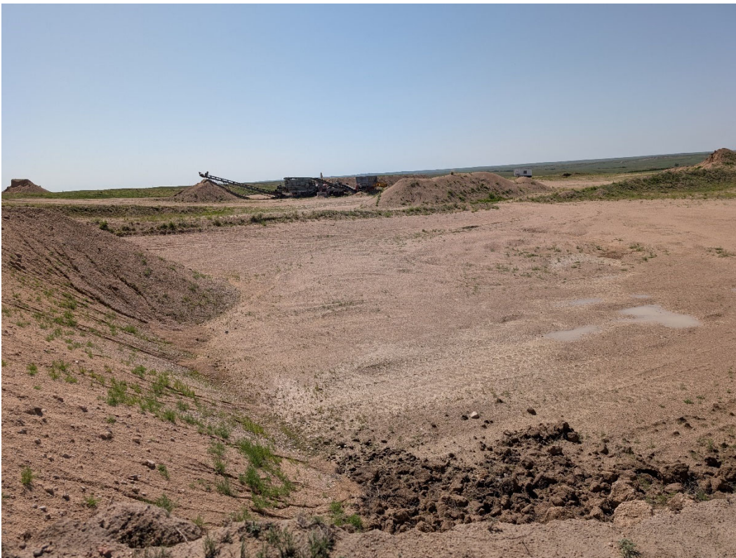
Photo 4: Looking southeast across the pit. Processing equipment observed in the middle of the pit floor. Slopes are 3H:1V here.
