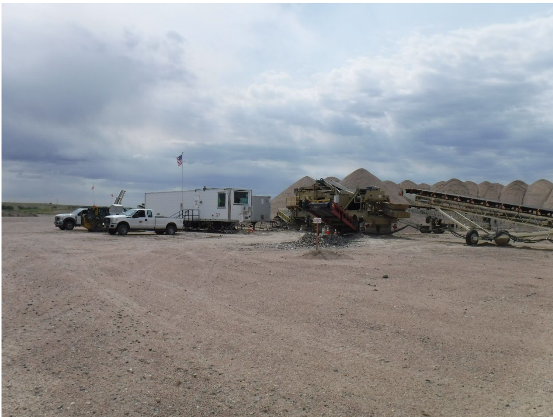
Photo 4: Portable screening and crushing equipment
