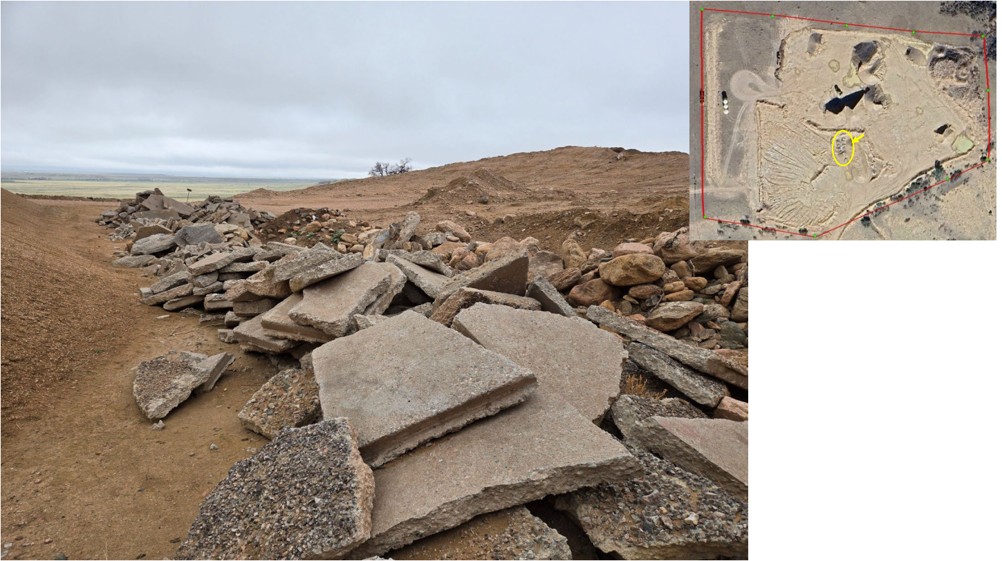
Photo 13: Stockpiled concrete stored onsite to be recycled into product.
