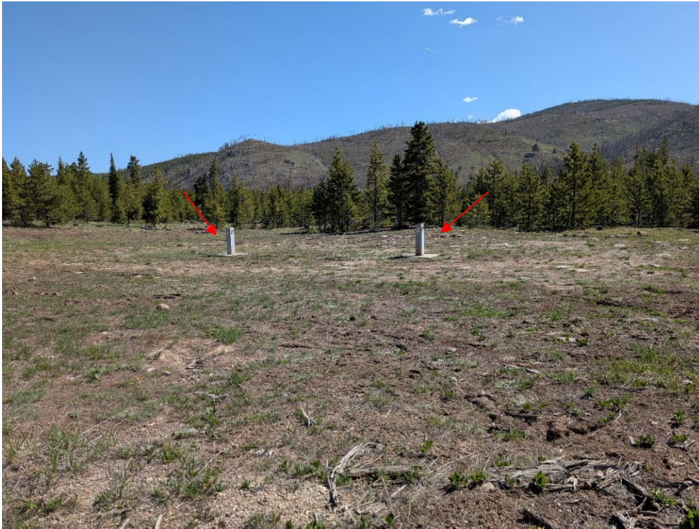
Photo 13: Looking east at two groundwater wells (MLGW-17 and MLGW-20) downgradient from the seepwater collection area.
