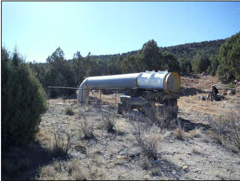
Figure 2. Overview of IF 5MN13751, a motorized air vent associated with the JD-5 mine, located on the north facing slope of Monogram Mesa, facing south-southeast.
