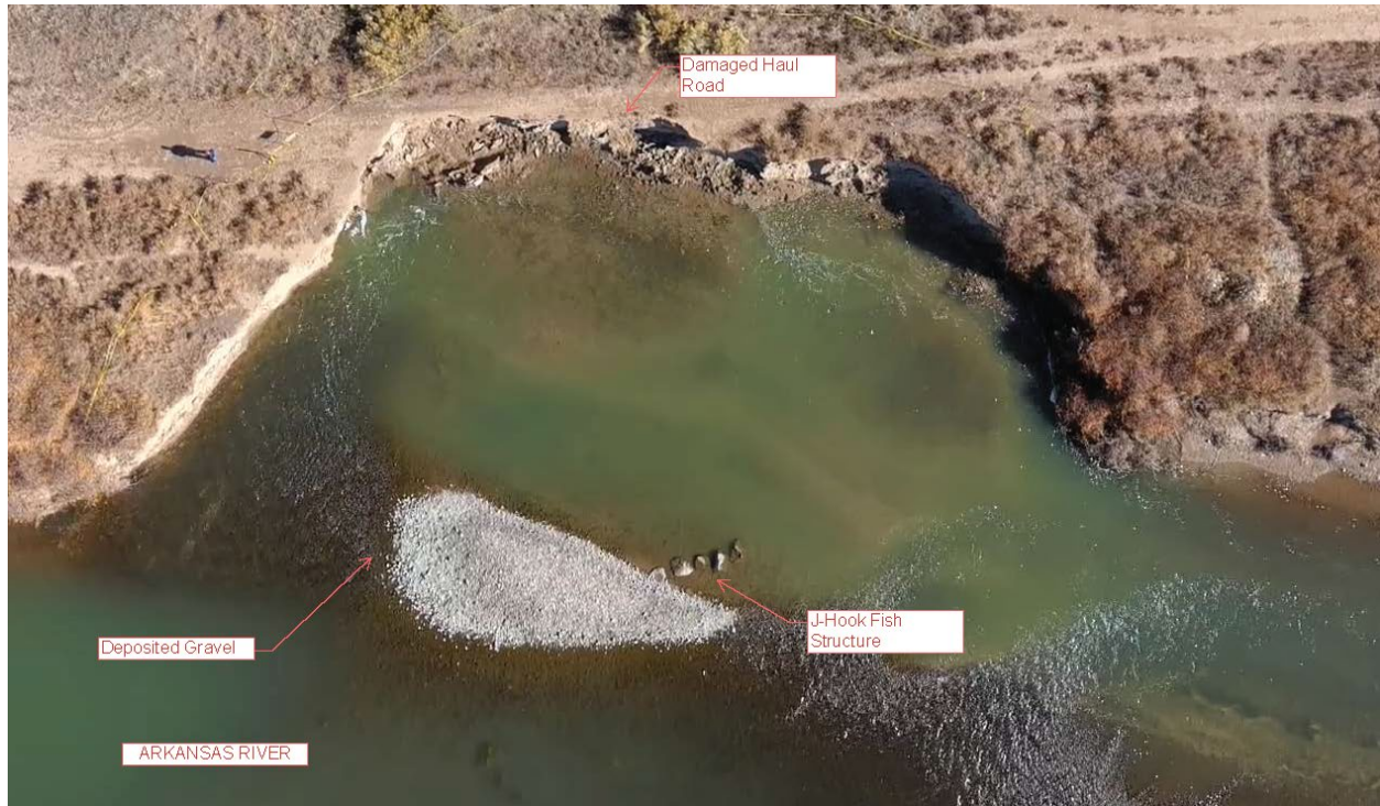
Figure 2. Overview of The Scour Hole at West Pueblo Pit, Showing Cause of Erosion and Damaged Areas.
