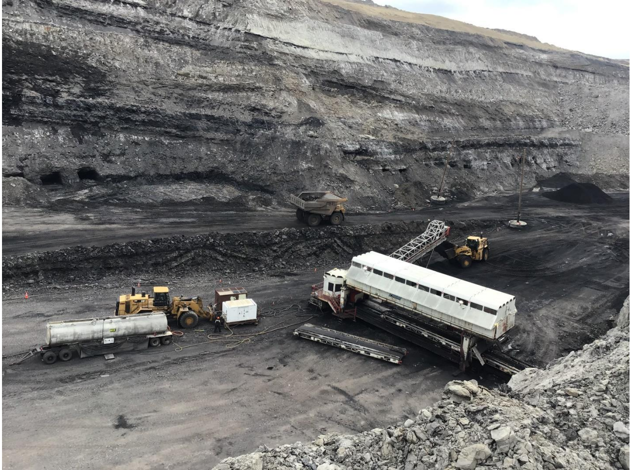
Photo 9: View of N Pit from above looking south. Coal is being produced by the highwall miner.
