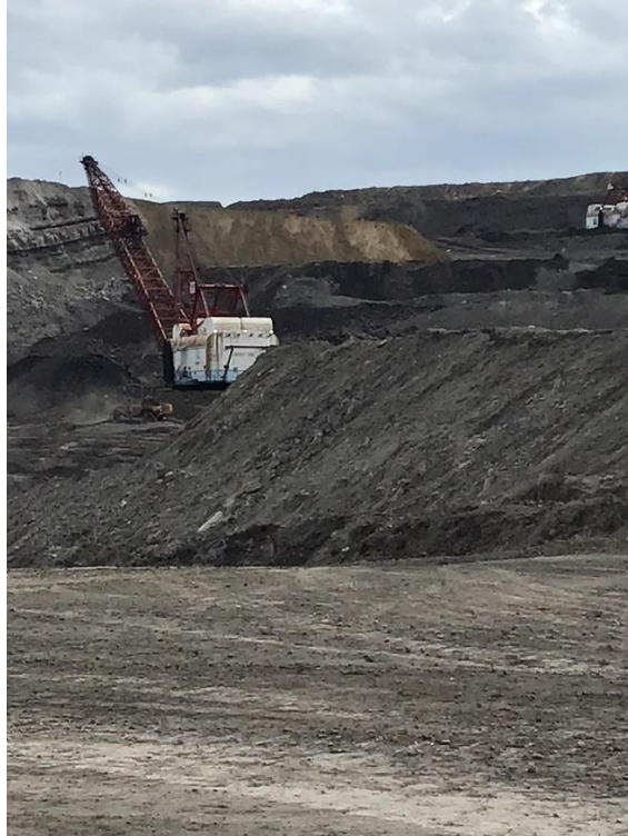
Photo 7: Drag Line working in L Pit, looking south.
