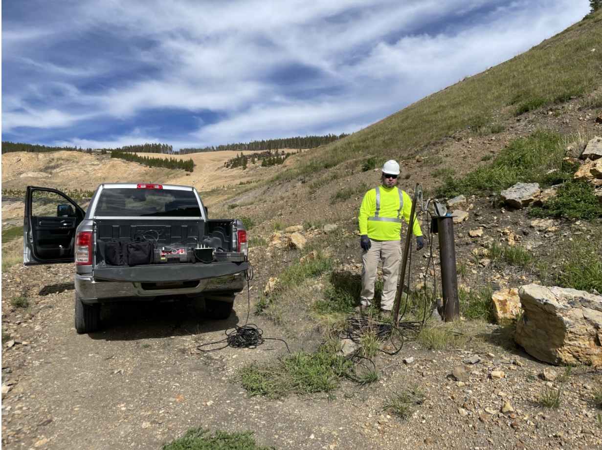
Photograph 1: Readings from inclinometer I98-1
