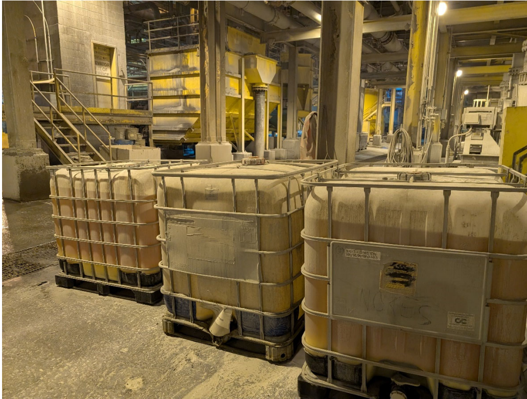
Photo 4: Mill EPF 2.3a - Frother Chemical Storage (Dowfroth 250-C) totes
