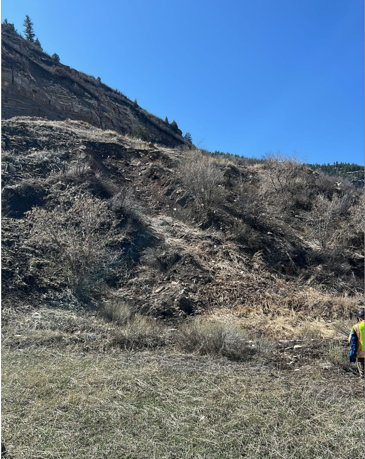
Figure 4: Slumped soil at groundwater seep
