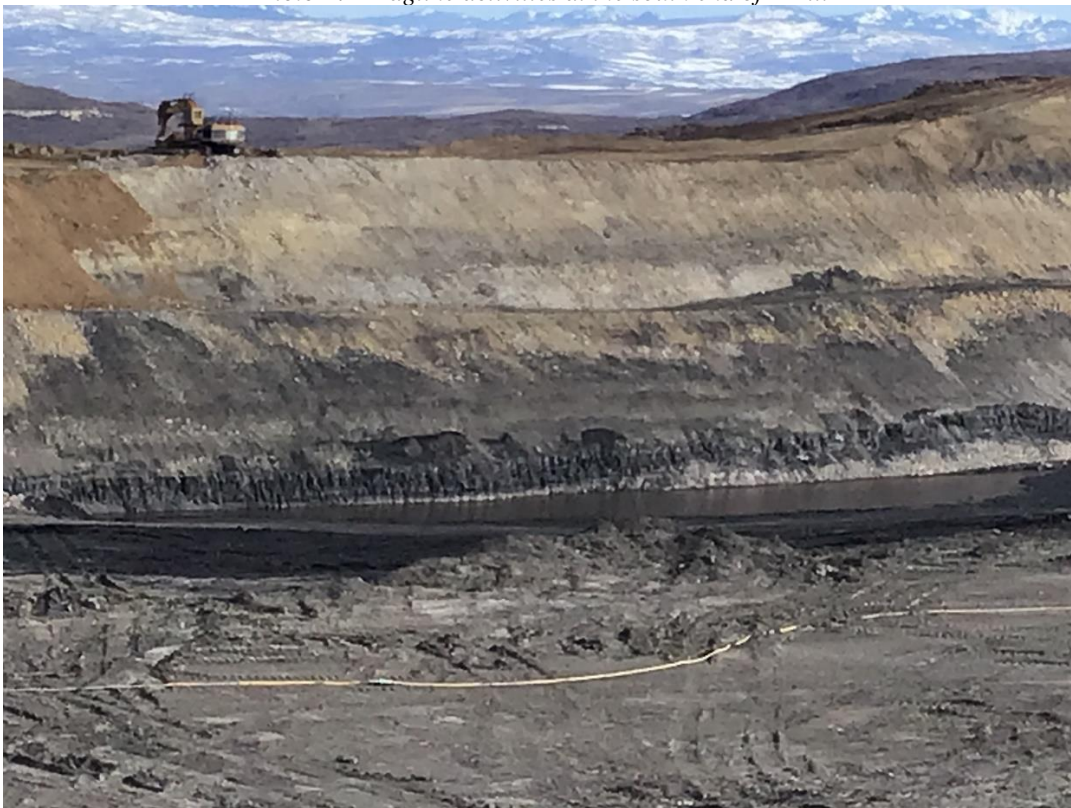
Photo 3: L Pit looking east. Water lying against the highwall.
