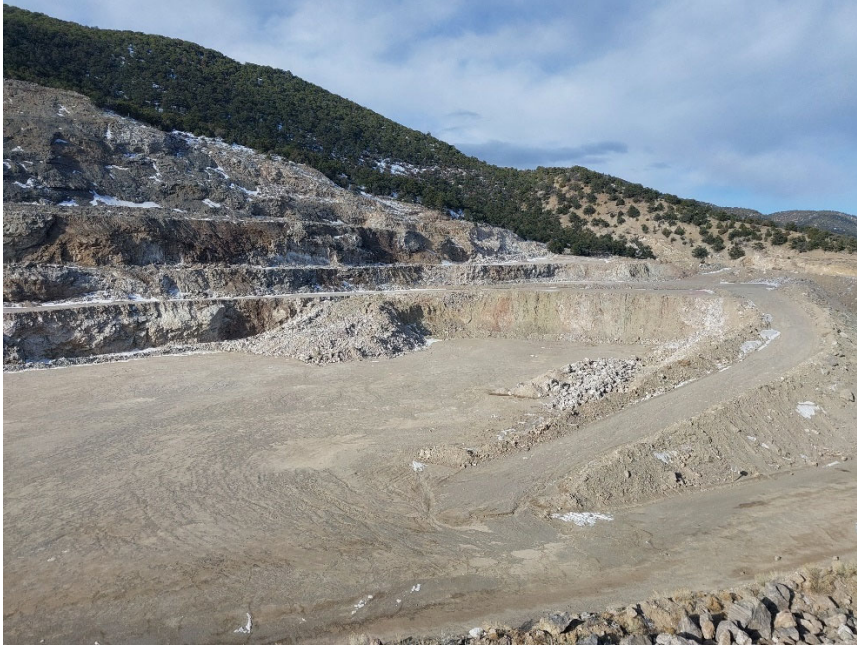
Photo #4: Quarry North, blasted material is stockpiled at the foot of the highwall on the pit floor. The three benches can be seen. Looking west-northwest.
