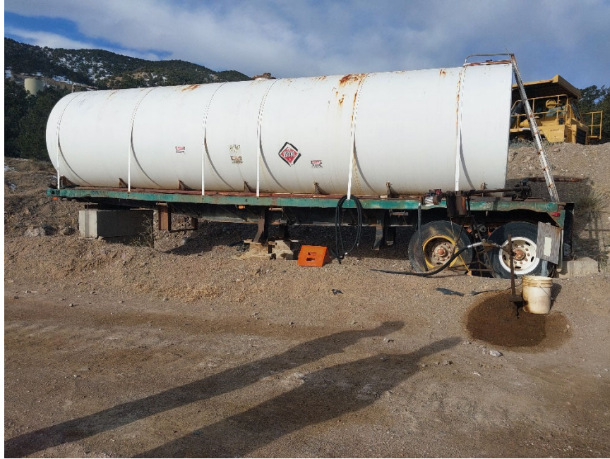
Photo #13: The portable fuel tank, the pump system and the post for the nozzle can be seen. At the base of the 5-gallon bucket, the discoloration of the ground indicates that the leak has been ongoing for some time and has spread.
