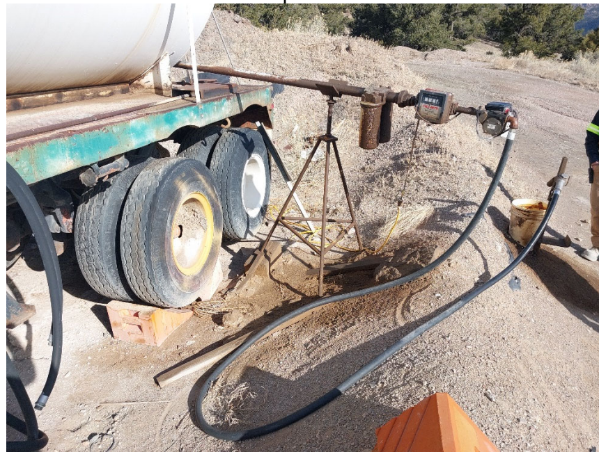
Photo #14: A closer look at the pump system on the fuel tank. The leak from the fuel/water separator can be seen on the separator and the ground below.
