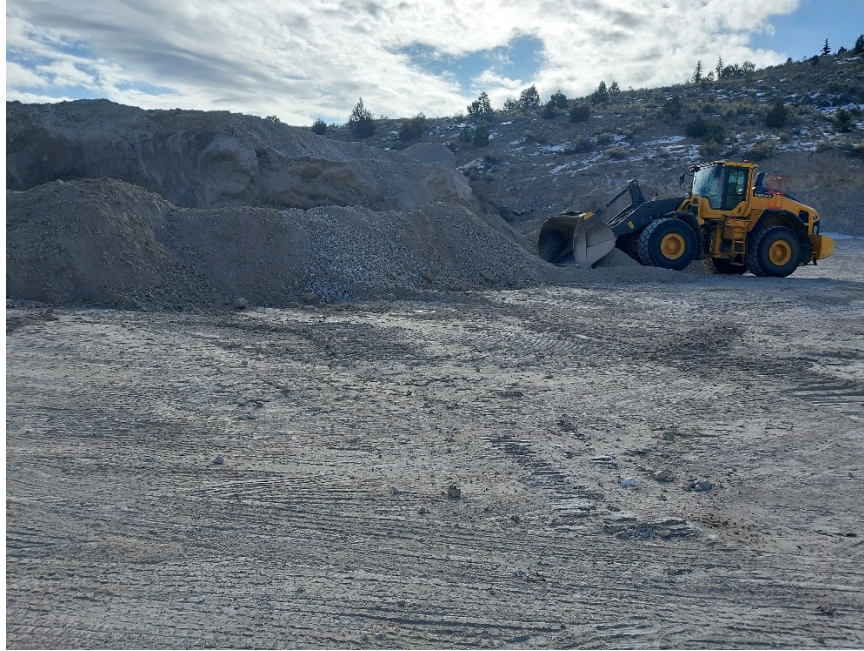
Photo #9: Product stockpile, tracks and freshly disturbance can be seen in the photo where material was loaded and hauled to the Portland Plant.
