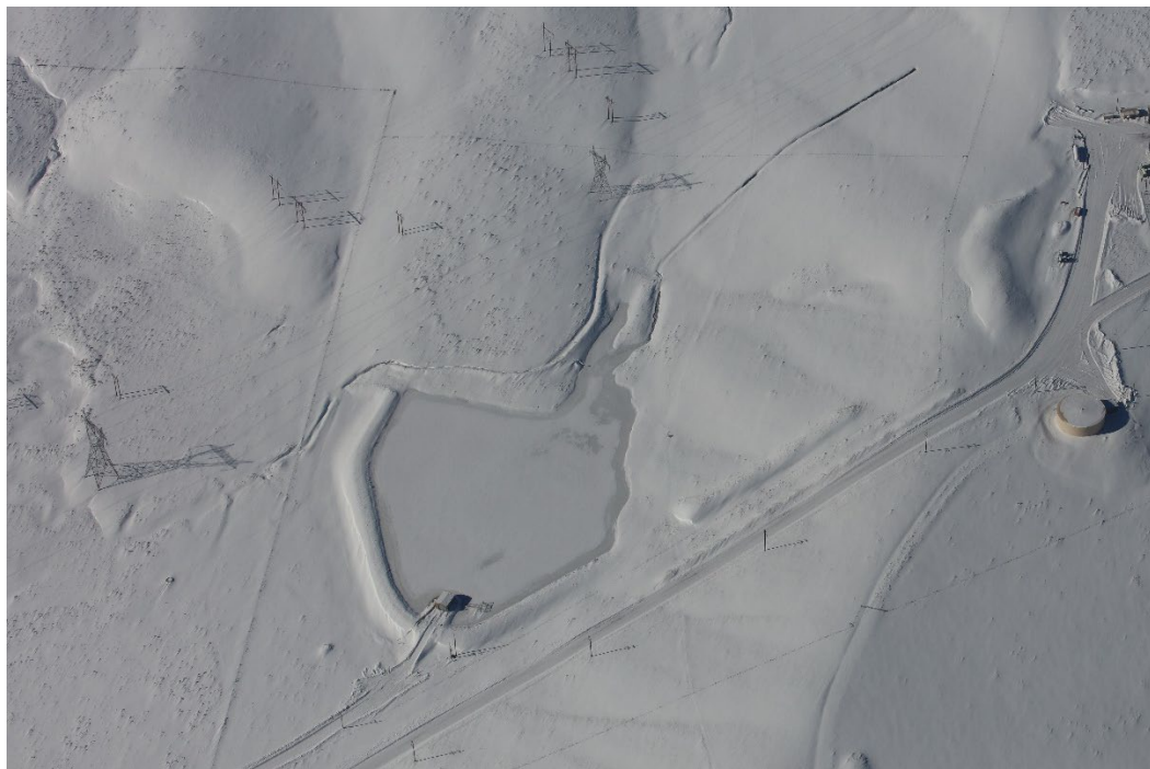
Photo 5- 6MN reservoir with inlet ditch in upper left
