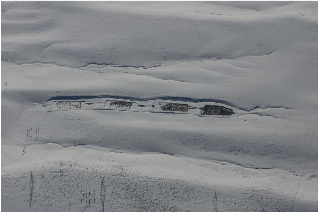
Photo 4- Four treatment pond near the 6MN facilities
