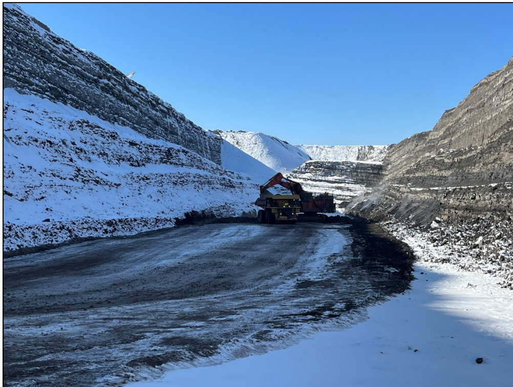
Photo 2: Spoil is being loaded from the central Collom Pit mining area and hauled to the eastern mined area.
