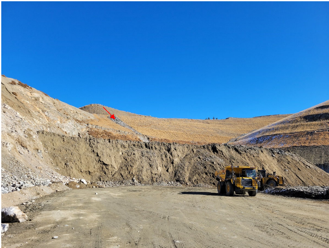
Photo 12: Mining in the northwest side of the permit area. Active mining is ongoing on this level. Slopes above have been reclaimed and an armored stormwater channel is noted by the arrow.
