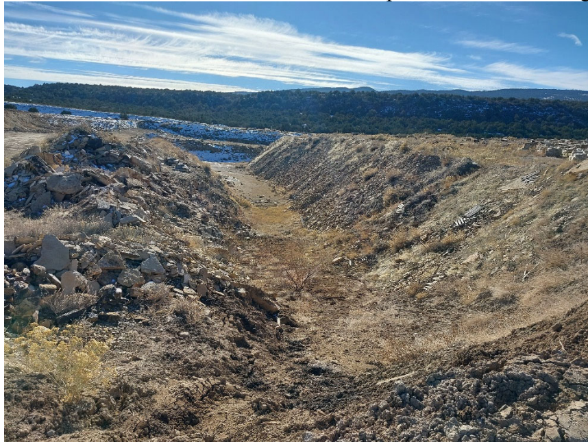
Photo #7: From the northern section of the permit area looking to the south-southwest. The bedrock Mine #1 highwall, the capstone layer above the gray clay, the Siloam Mine highwall, and the pit floor can be seen on the left side of the photo. On the right side of the photo, the area above the pit floor is used for storage of product material for the other two mines operated by Siloam Stone, Inc.
