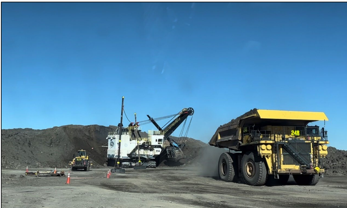
Photo 22: A shovel was observed to be filling haul trucks with spoil material in Collom Pit.
