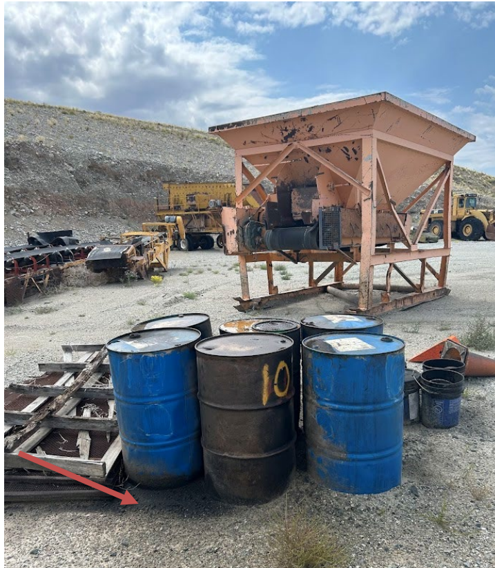
Photo 11: Oil drum (#1) with evidence of leaking within the North Area Pit.
