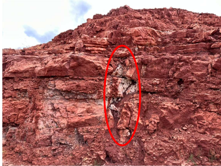
Figure 4: Silty/Clayey joint infilling along the secondary sub-vertical joint set outlined in red.
