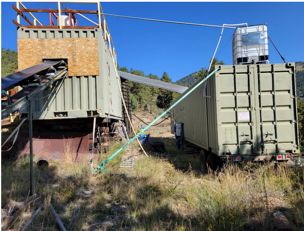
Photo 5: Looking north at the mobile Ball Mill Trailer on the left and Flotation Trailer on the right.
