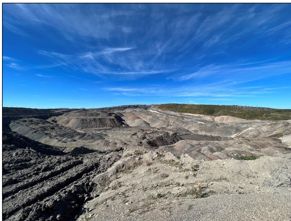
Photo 22: View into the South Taylor Pit, currently being backfilled, with continued benching in the southwest corner.
