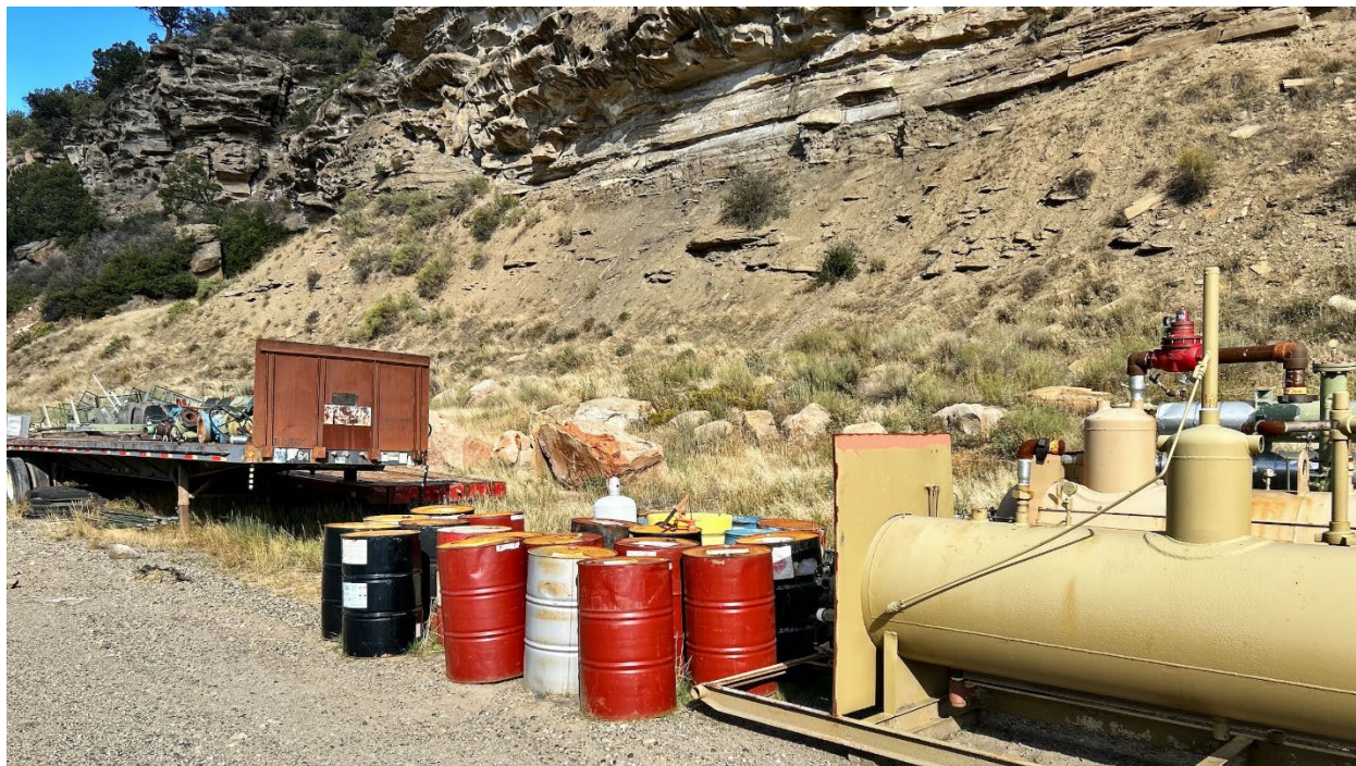
Figure 2: Unmarked steel drums, with no secondary containment (most, but not all, empty)
