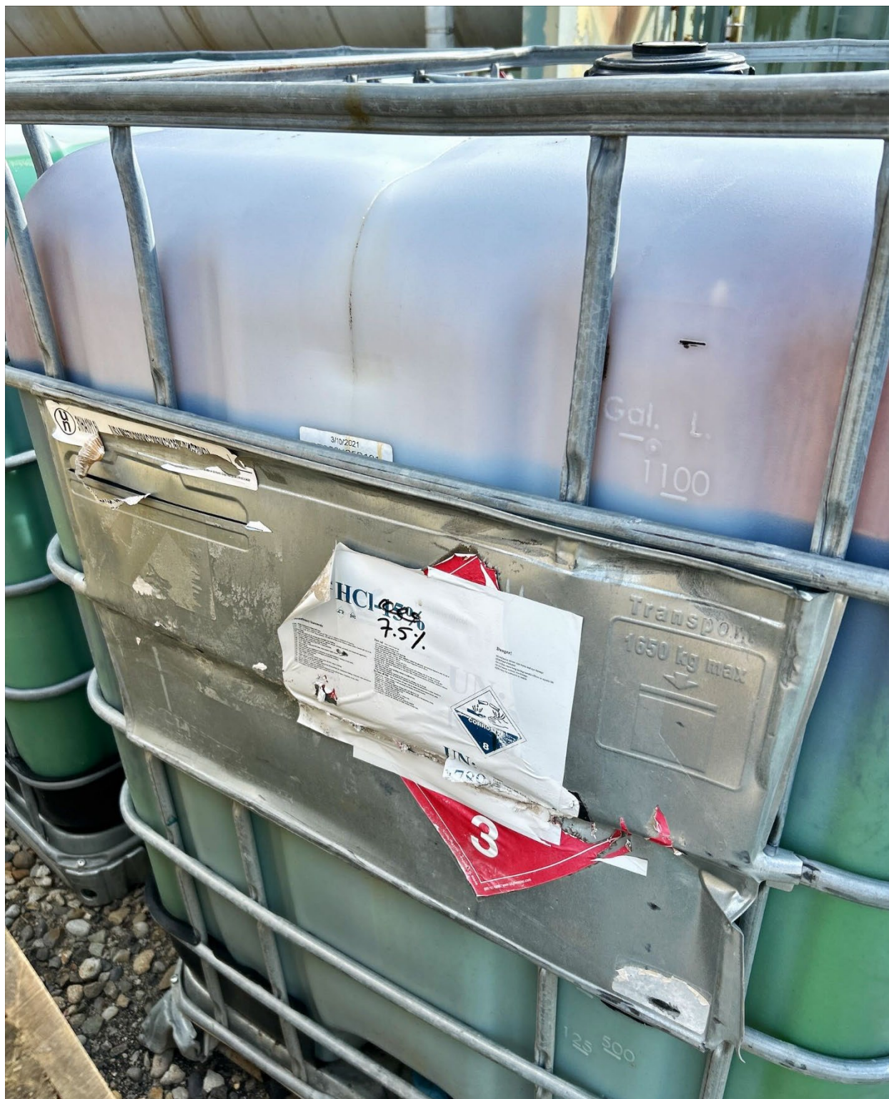
Figure 4: Tote labeled as Hydrochloric acid stored in East Yard, no secondary containment
